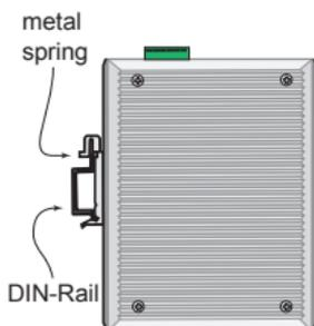
To remove EDS-505A/508A from the DIN-Rail, simply reverse Steps 1 and 2.
