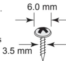
**NOTE** Before tightening the screws into the wall, make sure the screw head and shank size are suitable by inserting the screw into one of the keyhole-shaped apertures of the Wall Mounting Plates.
